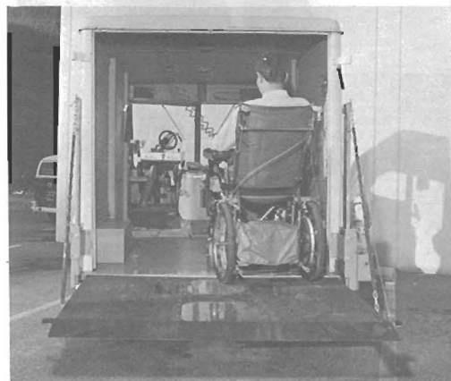
Wheel wells guide and position chair
